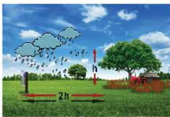
The top surface of the gauge should be horizontal and chest high; the grass and vegetation around it should be less than a knee high.
